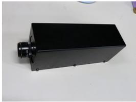
FIG. 10. Hyper-spectral camera HSC-1700 manufactured by Eba Japan Co., Ltd.
